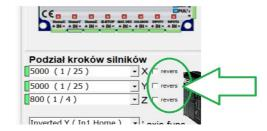
The next step is to determine the gearing parameters of individual axes.
