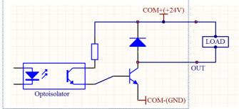
Figure IV switch output circuit
